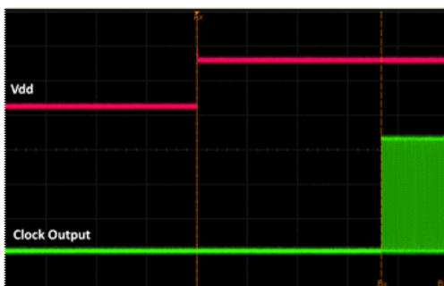
Figure 17. Startup Waveform vs. Vdd
